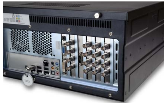
Server with video capture cards installed
